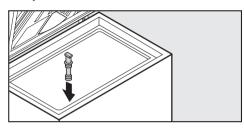
Use the stopper supplied to plug the defrosting outlet in the bottom of the interior of the appliance.
